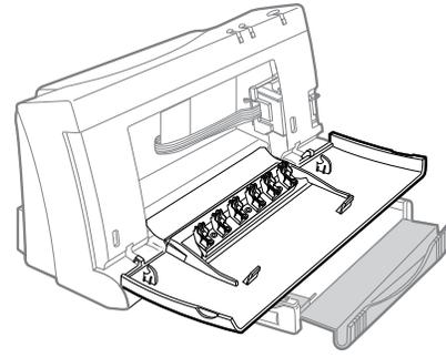
7. Turn on the printer. The carriage should move along the carriage path and return to the home position.
