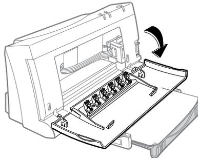
3. Look inside the printer and determine if the print cartridge and print cartridge cradle are in the home position (right end of the mechanism).
