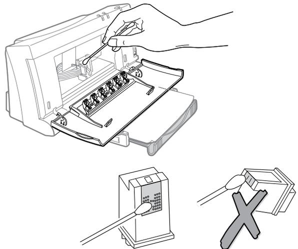
3. Once the print cartridge and print cartridge cradle contacts are dry, reinstall the print cartridge. Retest by printing the printer self-test.
