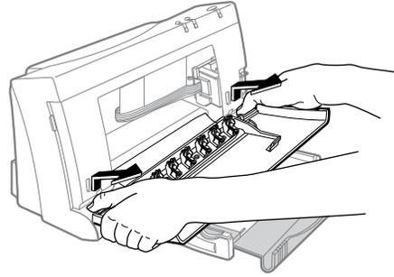
3. Open the paper separator (the flap that separates the printed pages from the blank sheets) by pulling it toward you.
