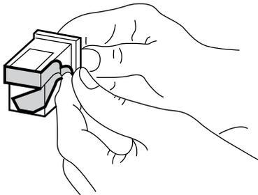
6. Insert the print cartridge into the holder at an angle such that the green top is tilted toward you. The arrow on the print cartridge should be pointing toward the inside of the printer.
