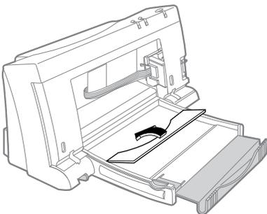
6. Close the printer door. Load paper and turn on the printer.
