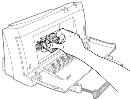
2. Remove the print cartridge from the printer and clean the print cartridge and print cartridge cradle contacts. Use a cotton swab lightly moistened with water. *Do not wipe the ink nozzles on the print cartridge.*
