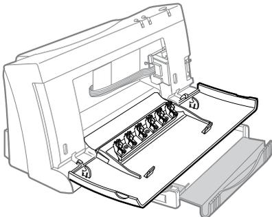
4. Turn the printer off. Because of the stall condition, the printer should turn off with the print cartridge out of the home position.
