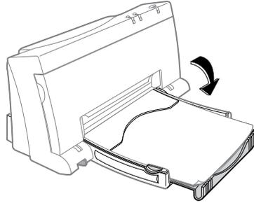
3. Open the printer door and switch the envelope lever to envelope if you are using envelope, labels or thick paper. Switch the lever to paper if you are using paper or transparencies. Then close the printer door.
