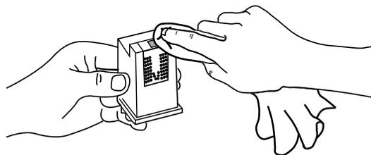
7. Repeat the above steps of installing the print cartridge, cleaning the print cartridge contacts, cleaning the print cartridge cradle contacts, and clearing the nozzles several times. If the problem consistently appears in the printer self-test with the same rows of dots missing on different print cartridges, return the printer for repair.
