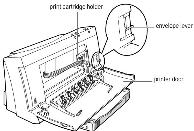
**Figure 1-2. The HP DeskJet 400 Printer (Internal View)**
