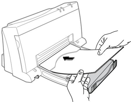
4. Move the paper width guide so that it presses lightly against the paper stack.
