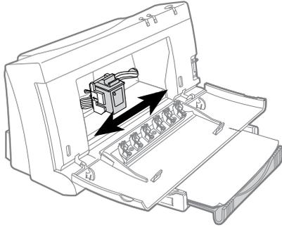
6. If the printer has a service station motor stall error condition, look for any visible obstructions around the service station (right end of the mechanism) that may be hindering the service station operation. If the problem cannot be resolved, return the printer for repair.
