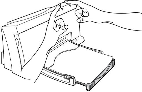
2. If you are using manual feed, insert a sheet of Letter- or A4-size paper in the paper feed slot.
