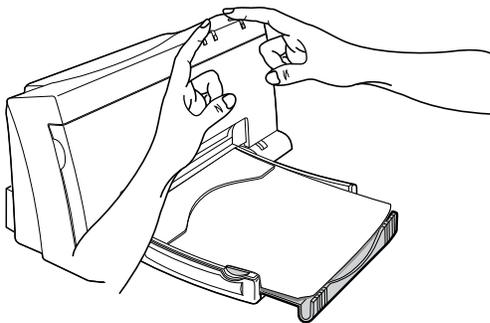
4. If using the printer manually, load a sheet when the Paper Feed light starts blinking. See "Loading Media" in chapter 3 for instructions on manually loading paper.
