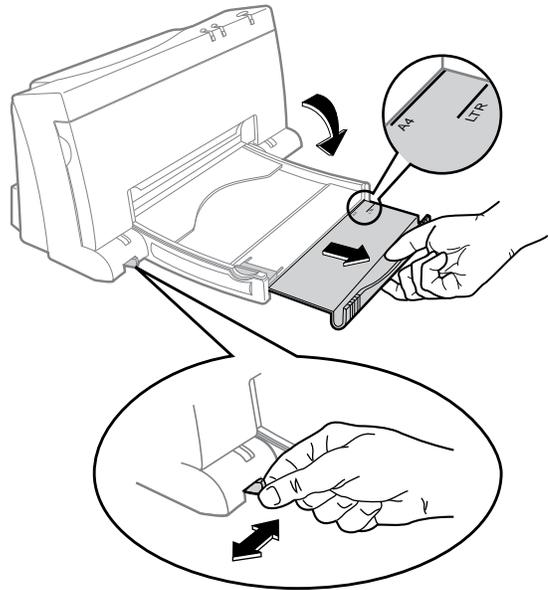
3. Insert a stack of paper into the paper tray with the print side down. If you are loading letterheads or HP transparencies, insert them print side down, with the top of the page going into the printer.
