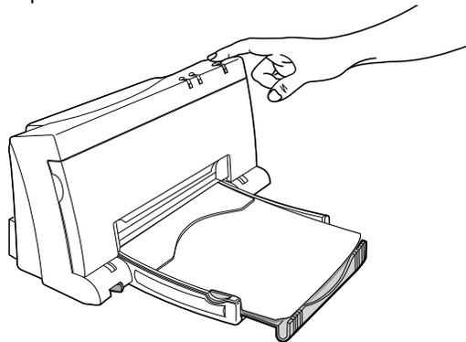
5. If the printer has a carriage stall error condition, look for obstructions or binding along the printer carriage path. Slide the print cartridge cradle back and forth across the printer mechanism. If the problem cannot be resolved, return the printer for repair.
