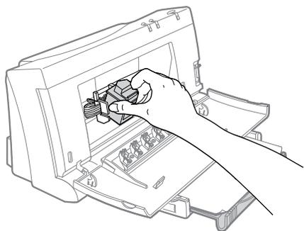
4. The print cartridge may be faulty. Replace the print cartridge and retest by printing the printer self-test.
